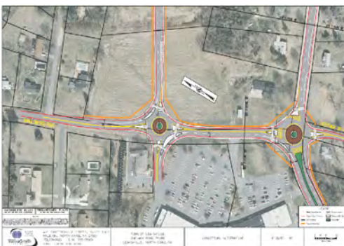
Roundabouts are proposed at Shallowford and Williams Roads and the parallel road facility.
