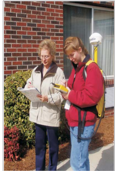
Winston-Salem DOT staff use the GPS Unit backpack to collect data on the sidewalks.
